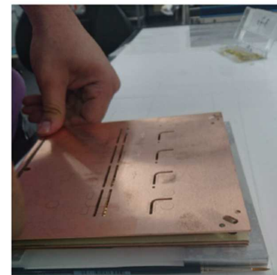
Fig. 7: Final deposition of the upper plate (negative supply plan)
