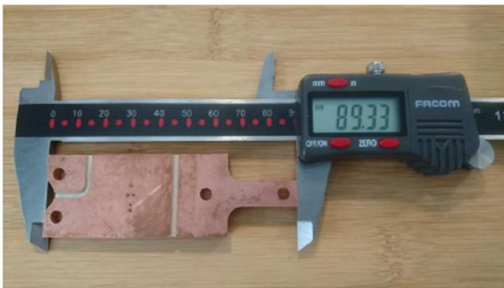
Fig. 10: Bottom view of the final module (calliper measurement in mm)
