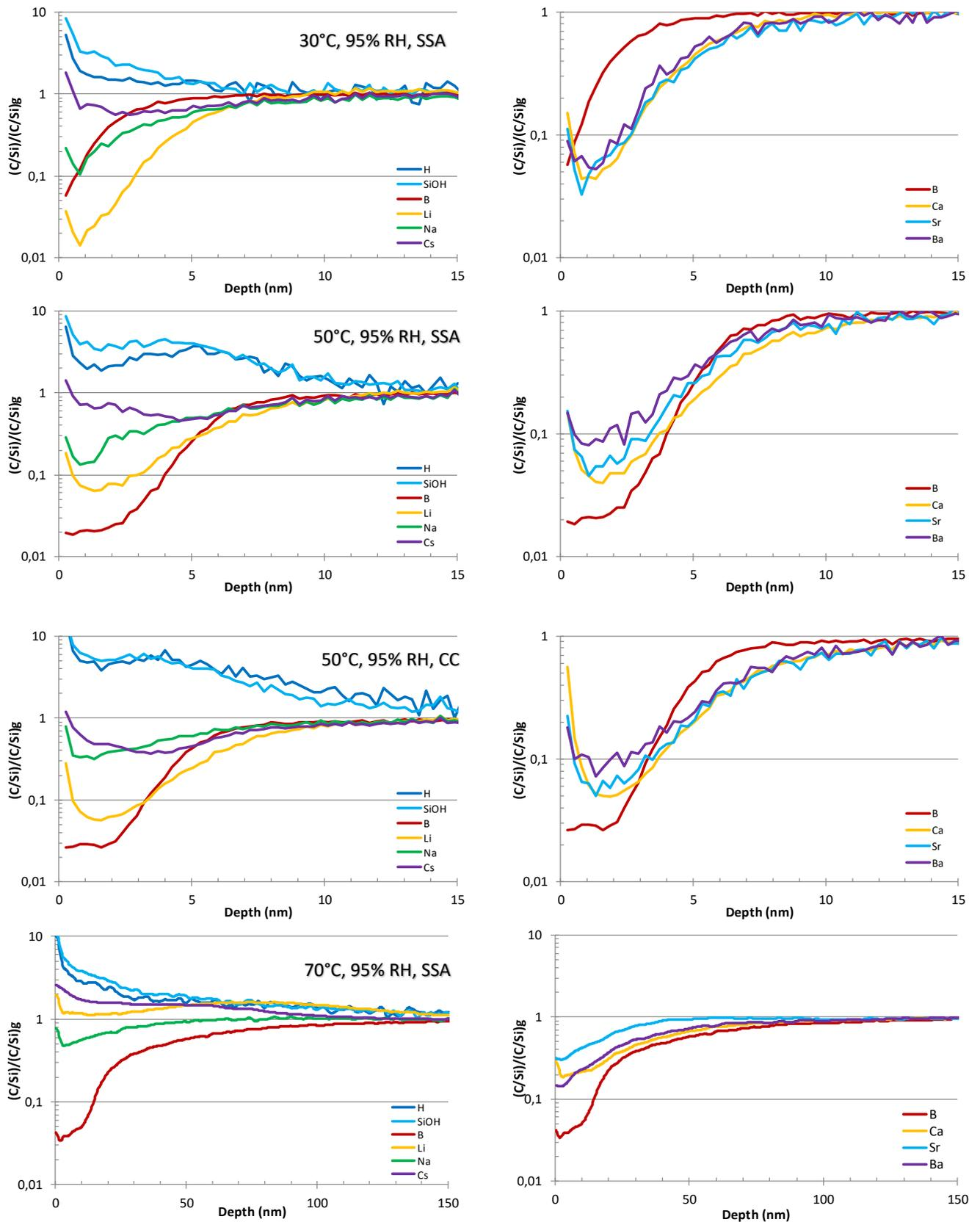
Figure 1: Elemental TOF-SIMS profiles for SON68 glass hydrated over 6 months at 30, 50, 70 °C, and 95% RH. From top to bottom: Test 1: 30°C (Stainless Steel Autoclave), Test 2: 50°C (SSA), Test 4: 50°C (Climatic Chamber), Test 6: 70°C (SSA).
