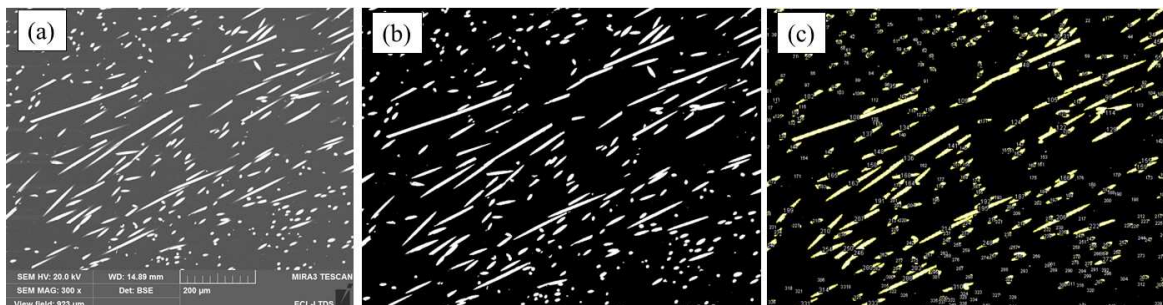
Fig. 3 Image analysis process: (a) Obtained SEM image; (b) binarized image; (c) image showing particle analysis.
