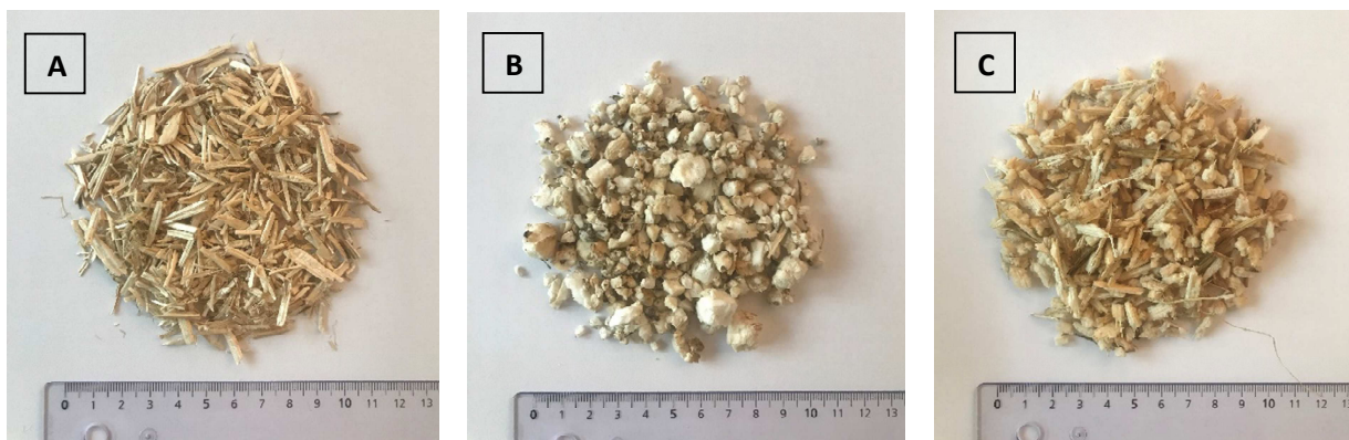
34 Fig. 1. Aggregates used in this study (A) Hemp shiv, (B) Sunflower pith and (C) Maize pith
