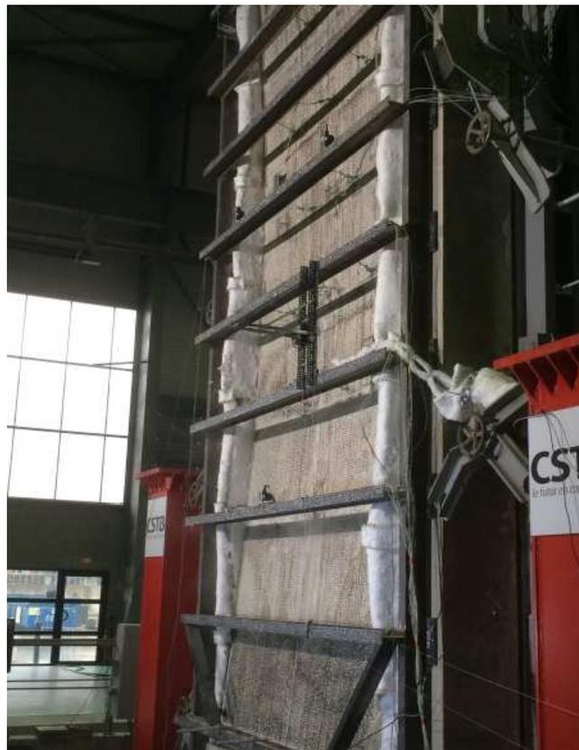
**Fig. 8.** Deformed shape of the wall after 90 min of fire exposure time
