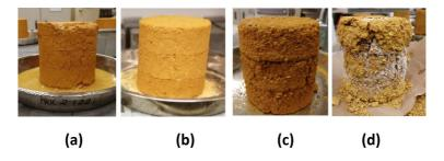
**Fig. 7.** Evolution of damage on the unstabilized sample PROC-US-MR-FT after (a) 1 cycle, (b) 2 cycles, (c) 3 cycles and (d) 4 cycles
