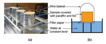
Fig. 3. Illustration (a) and schematic presentation (b) of the setup for water absorption test
