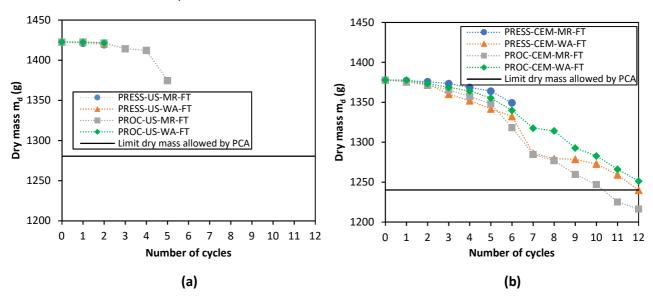
**Fig. 11**. Evolution of dry mass of unstabilized samples (a) and stabilized samples (b) exposed to freezing-thawing cycles
