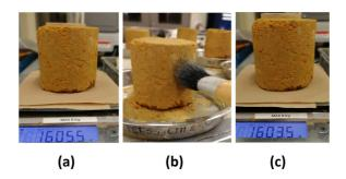
**Fig. 5.** Procedure for assessing mass losses by scaling: (a) first weighing before brushing the sample, (b) brushing the surface to remove the scaled particles and (c) final weighing after brushing the sample.
