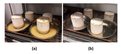
Fig. 6. Tested samples (a) with and (b) without water absorption by capillarity.
