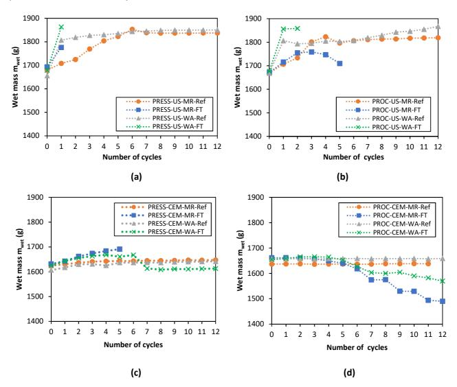
**Fig. 9.** Change in wet mass on PRESS (a), PROC (b), PRESS-CEM (c) and PROC-CEM (d) samples with number of cycles
