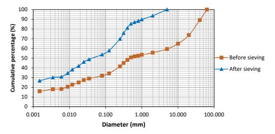
Fig. 2. The grain size distribution of the tested soil
