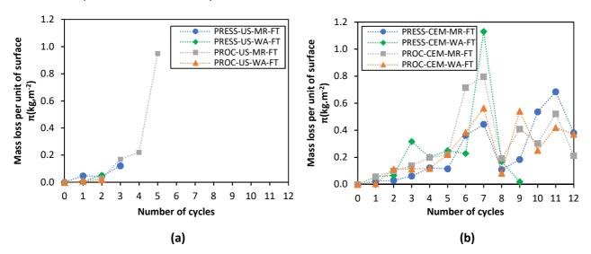
**Fig. 10.** Mass losses per unit of exposed surfaces of (a) unstabilized frozen samples and (b) stabilized frozen samples
