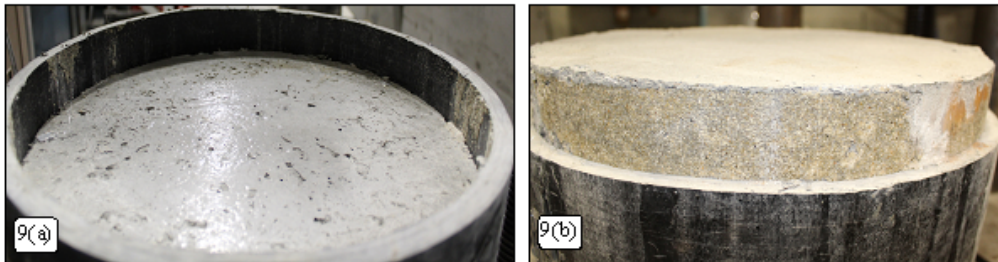
Figure 9: Specimens S-304-S after failure: (a) The interior surface FRP-T approximately smooth, (b) The sand-coating layer has completely stuck in the CC.
