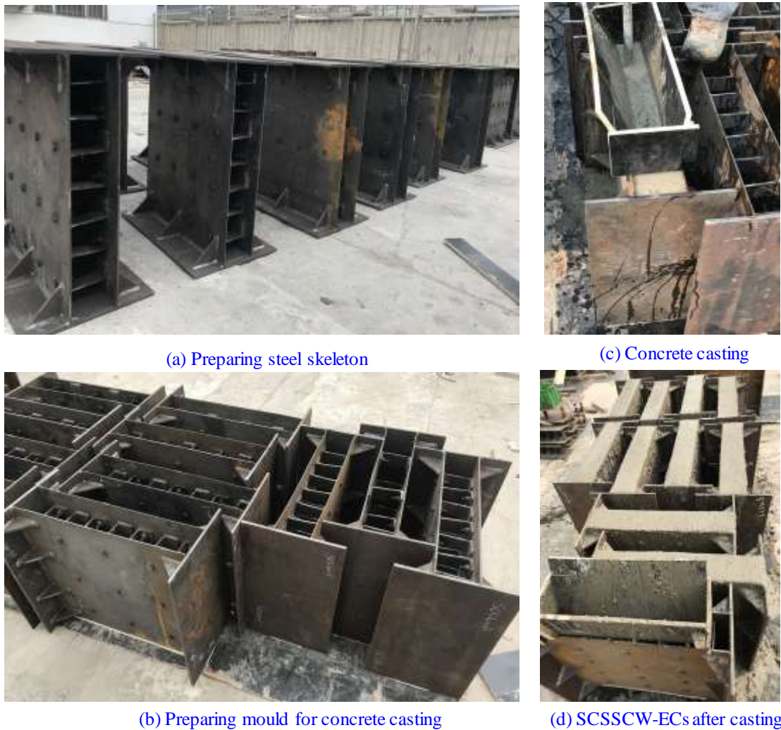
Fig. 3 Fabrication of SCSSCW-ECs specimens for testing
