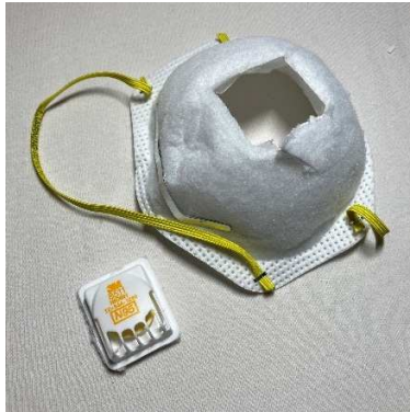
Figure 14. 3M Cool-Flow Exhalation Valve removed from mask.
