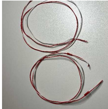
Figure 10. Controller cables; cut to length, stripped, and marked.
