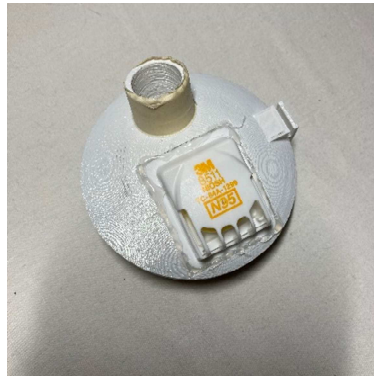
Figure 17. Apply tape to the nozzle to provide an air-tight fit to the hose.
