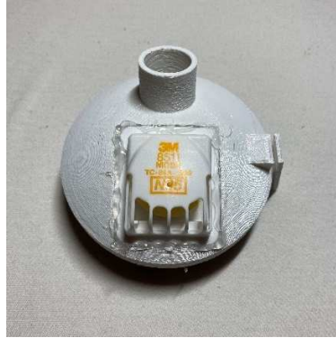
Figure 16. Glued 3M Cool-Flow exhalation valve in place.
