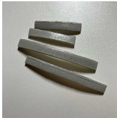
Figure 13. Weather-seal gasket, cut in half lengthwise.
