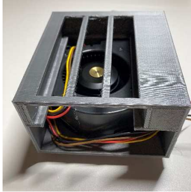
Figure 20. Properly run wire management.
