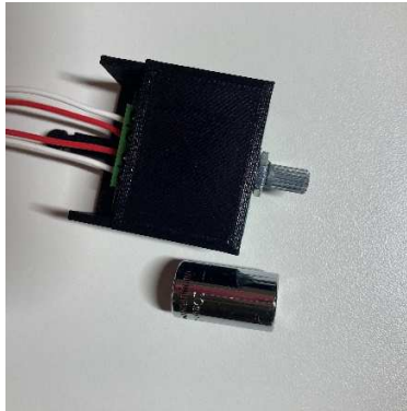
Figure 24. Fix the PCB into the controller case.
