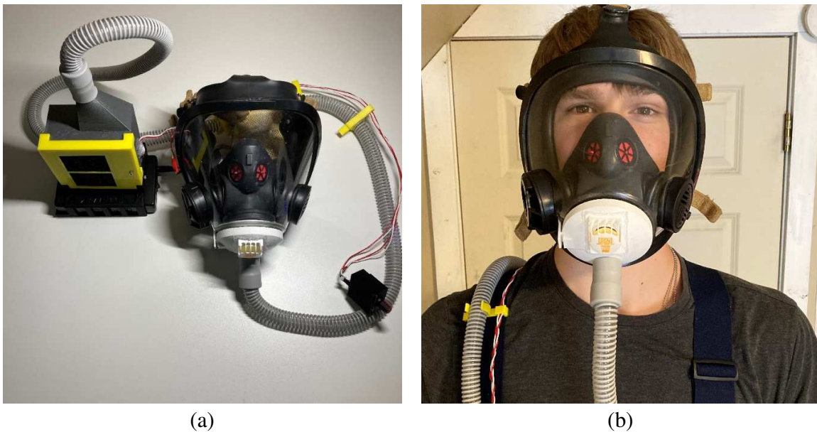
Figure 1. Fully assembled open source PAPR a) all components and b) in use.
