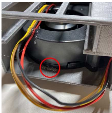
Figure 19. Glued fan in place (if necessary).
