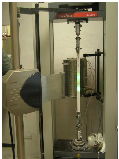
154 Figure 1. (a) Composite specimen; t , w , L : thickness, width, length of the specimen.; (b) Used “ball joint” 155 loading head; (c) Thermomechanical machine TM20kN-1200C; (d) furnace with specimen installed for a 156 thermomechanical tensile test
