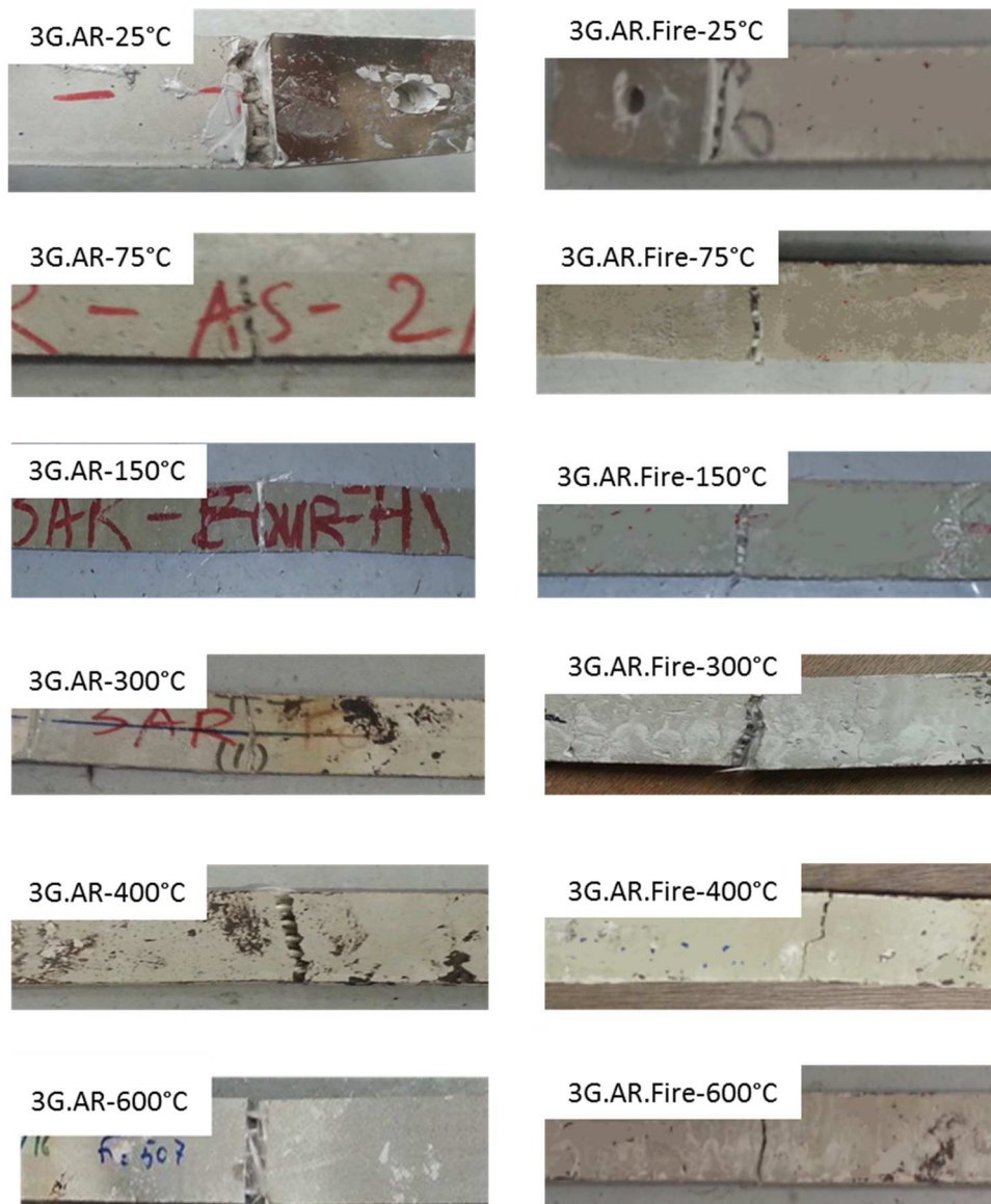
370 Figure 11. Failure modes of 3G.AR and 3G.AR.Fire at different temperatures
