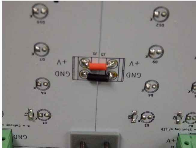
Figure 8. Wires directly soldered to transfer power from one board to the next
