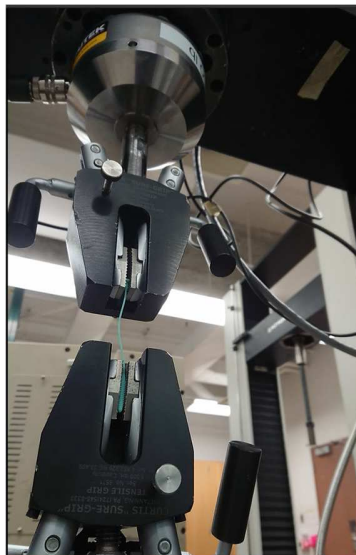
Figure 25. Mechanical testing of swabs with an Instron 4206.
