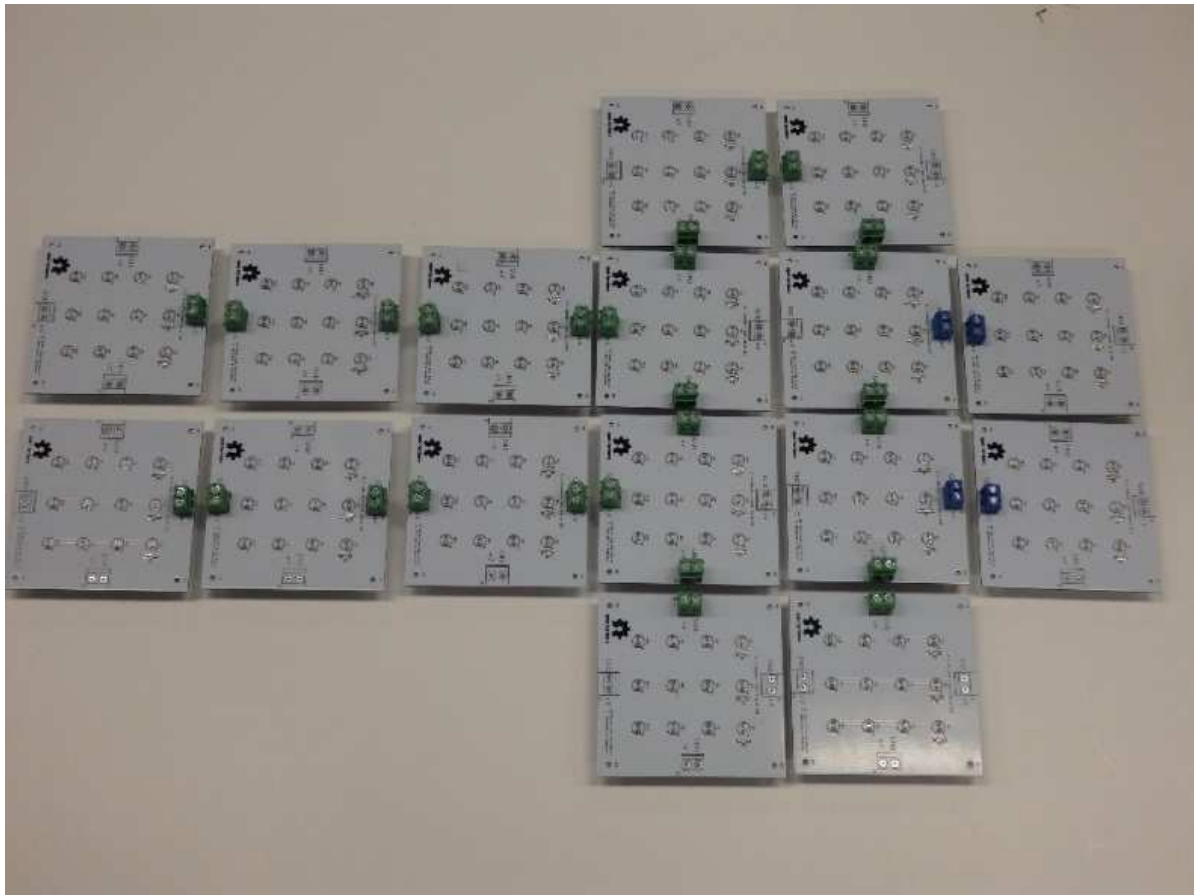
Figure 7. The UV curing box is first laid out in order to determine terminal block placement.
