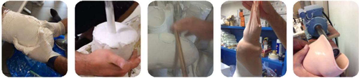
Figure 1: Current practice in the fabrication of the prosthetic socket
