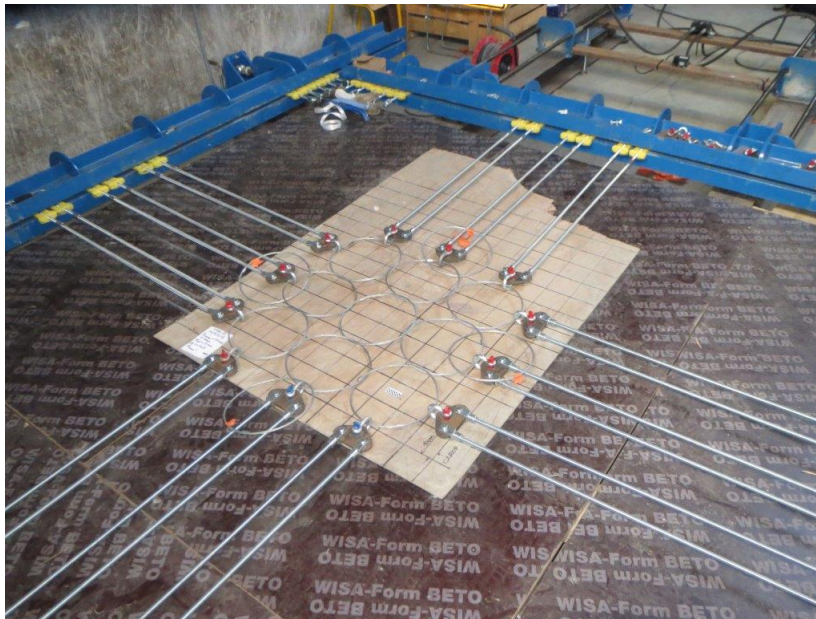
Figure 19: Experimental setup of the plane tensile test on a ASM4 ring net (Courtesy of PN C2ROP).
