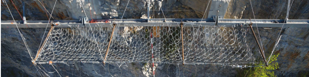
Figure 1: Top view of the rockfall barrier prototype developed in the framework of the french national project C2ROP (Photo courtesy of NP C2ROP).
