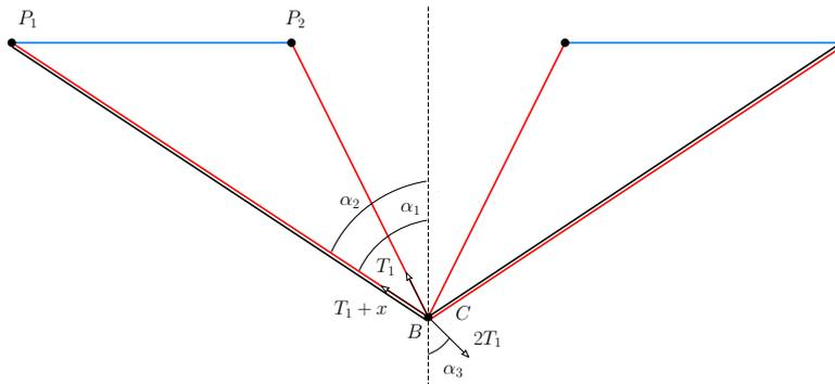
Figure 15: Limit equilibrium with a very low stiffness of the bar.
