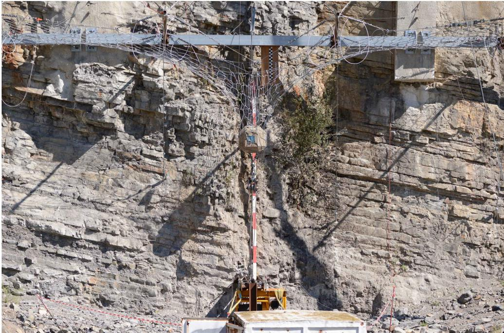
Figure 18: Front view of the quasi-static experiment on the rockfall barrier prototype (Courtesy of PN C2ROP).
