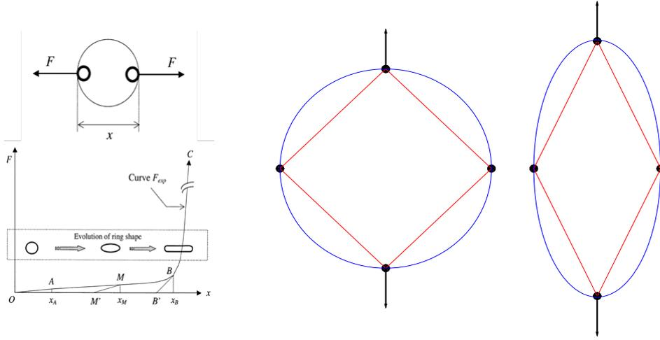
Figure 8: Experimental tensile test [22] and discrete ring model.
