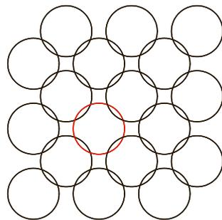
Figure 2: Pattern of a ASM4 ring net.
