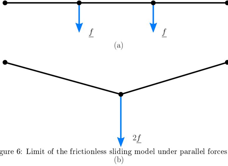
Figure 6: Limit of the frictionless sliding model under parallel forces.
