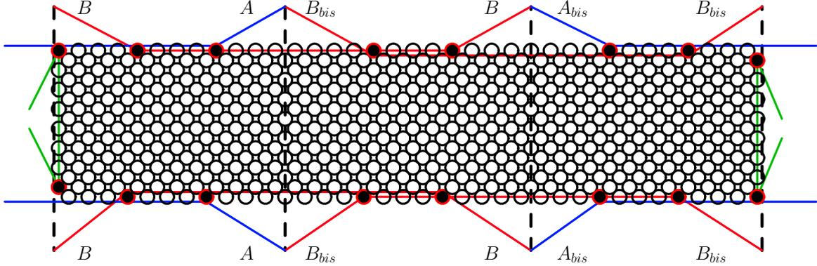
Figure 17: Support cables nomenclature and weaving principle scheme.
