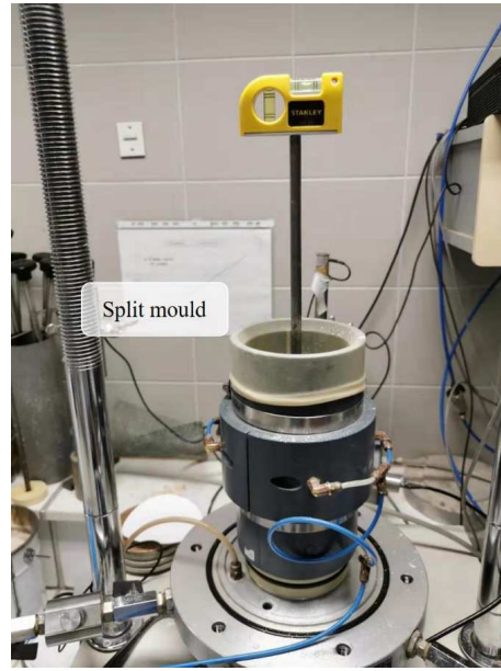
Figure 3 Dry tamping method (a) spooning the mixture into a split mould; (b) horizontality of each layer after slight compaction
