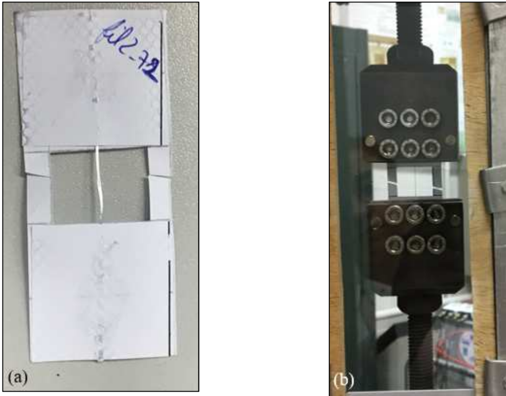
Figure 1. (a) Picture of a tested sample; (b) Picture taken through the window of the furnace, of a sample set up on the test machine
