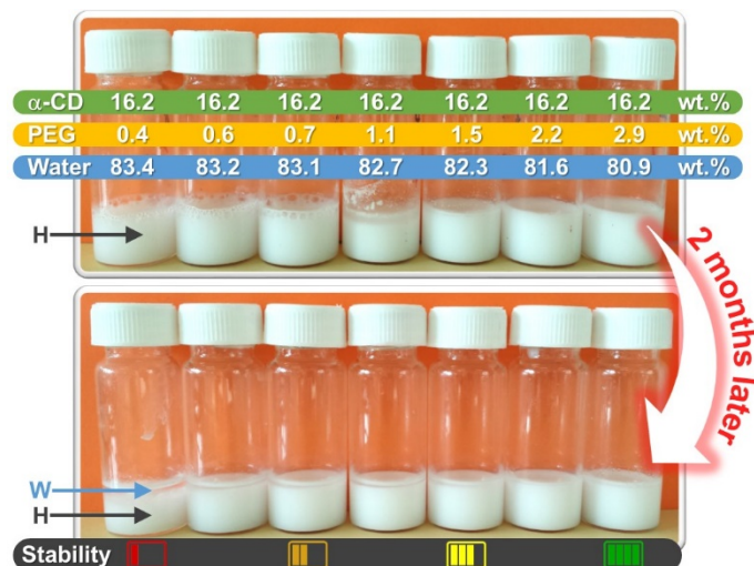
Figure 2. Photographs of various hydrogels prepared from aqueous solutions of \alpha -CD and PEG 20 000 at t = 0 (top) and 2 months (bottom, H = hydrogel phase and W = water phase).
