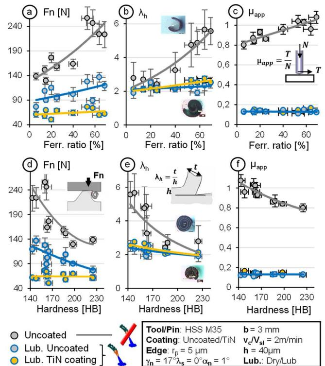
**Figure 4.** Influence of ferrite ratio and hardness on the normal force  $F_n$  (a,d), chip thickness ratio (b,e) and apparent friction coefficient (c,f) under dry and lubricated conditions.
