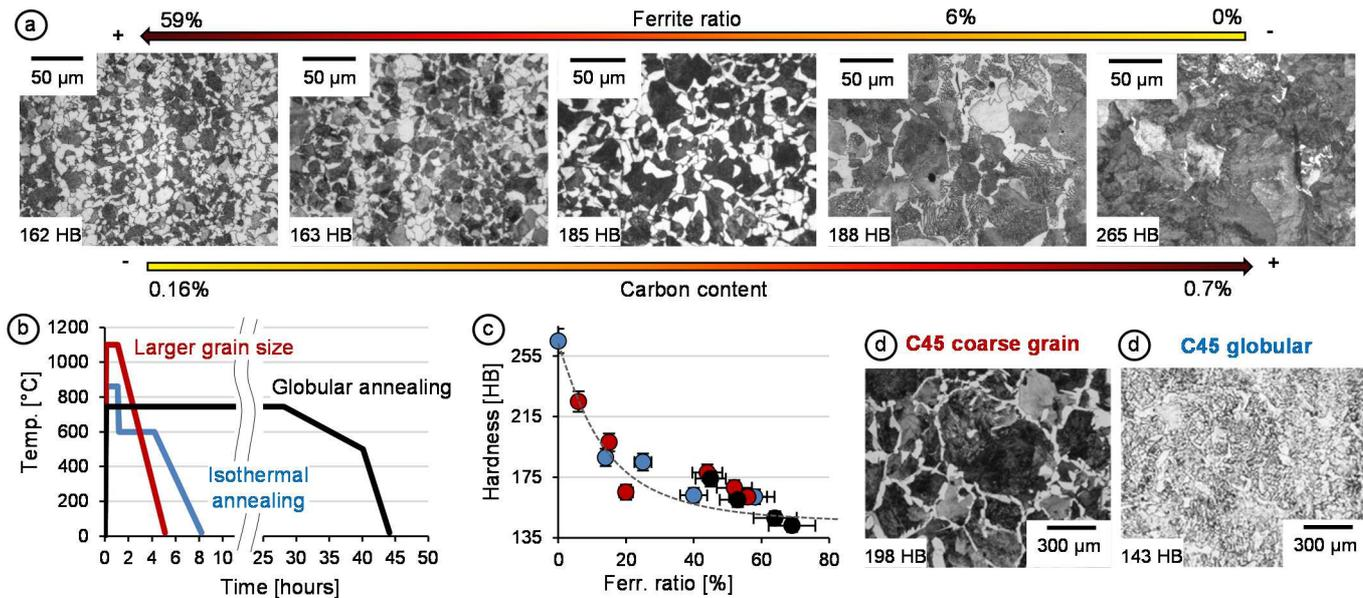
**Figure 1.** a) Examples of microstructures obtained when increasing the carbon content/ferrite ratio, b) heat treatment cycles applied to generate the various FP microstructures, c) correlation between ferrite ratio and macroscopic hardness and d,e) examples of corresponding micrographs when applying the heat treatment cycles to C45.
