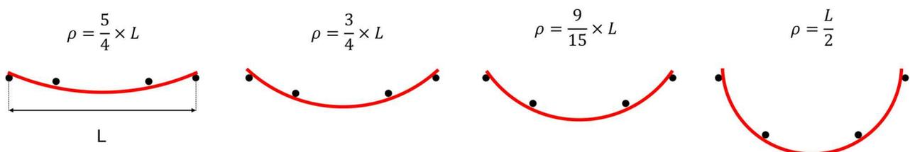
Fig. 5 Schematic illustration of the decrease of the bending radius during a four-line bending test
