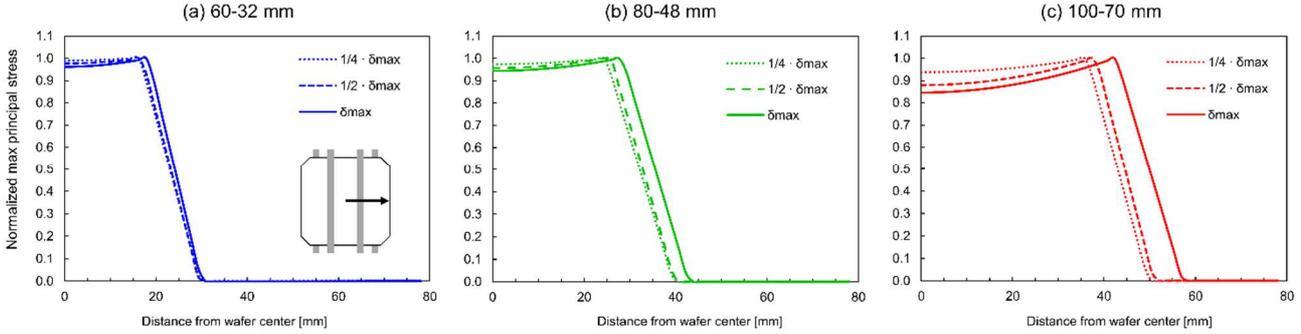
Fig. 11 Normalized maximum principal stress at the bottom surface and along the wafer length obtained by FE simulations for a given thickness (180  $\mu\text{m}$ ) and different displacement values for the configurations (a) 60-32 mm (b) 80-48mm (c) 100-70 mm
