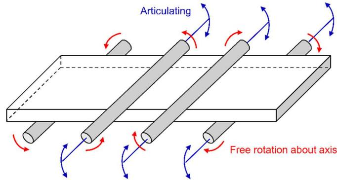
Fig. 8. Schematic figure of a fully-articulated bending fixture according to [7]. The two loading rollers are free to roll and they can independently articulate to match the wafer top surface. The two loading rollers are free to roll, and one can articulate to match the wafer bottom surface.
