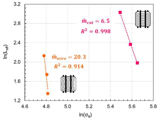
Fig. 14 Correlation between characteristic strength and effective length and evaluation of the mean Weibull modulus for each testing direction (least square method)
