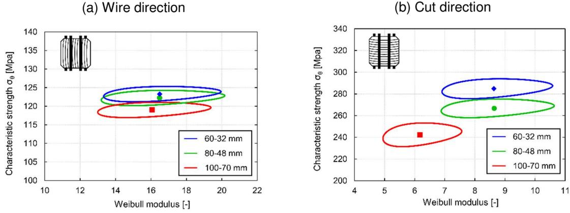
Fig. 13 Weibull 90% confidence contour plots for the three configurations in (a) wire direction and (b) cut direction
