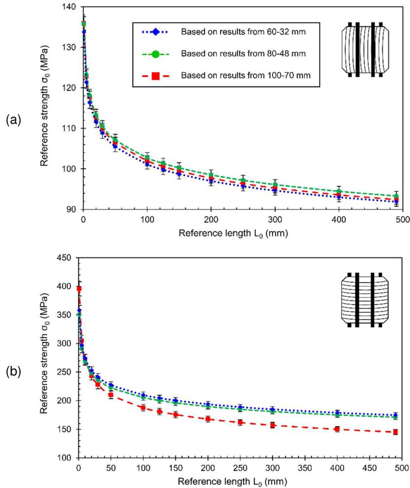
Fig. 15. Strength scaling laws predicting the evolution of reference strength  $\sigma_0$  as a function of reference length  $L_0$  in (a) wire direction and (b) cut direction based on results obtained with the three configurations
