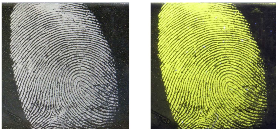
Fig. 18: Typical fingerprint developed with Lumicyano®. Left, under visible daylight; right, under UV (365 nm broad band) illumination.
