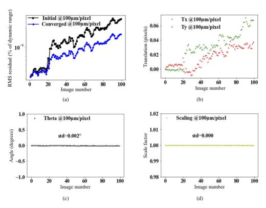
**Fig. 5.** Measurement results for the image set at low resolution (100  $\mu$ m/pixel) to estimate uncertainties. (a) RMS residual between the reference image 0 and all images of the set before correction and after image registration. Measured translations (b), rotations (c) and scale factor (d) as functions of image number.
