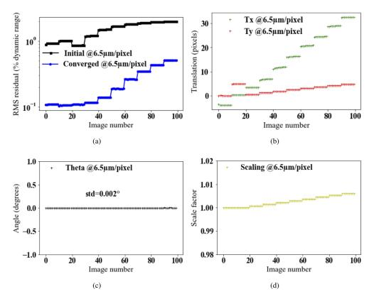
**Fig. 6.** Displacement measurements for an image set with a resolution of 6.5  $\mu$ m/pixel. (a) RMS residuals before correction and after image registration. Measured translations (b), rotations (c) and scale factor (d) as functions of image number.
