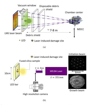
**Fig. 1.** (a) MDCC image acquisition setup at LMJ with the path of the laser beam shown in purple dash-dotted line. (b) MELBA experimental setup with the spatial shape of two available nanosecond ultraviolet laser beams.
