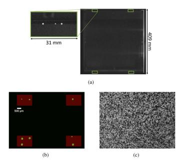
**Fig. 2.** (a) MDCC vaccum window image with fiducials in green boxes. (b) MELBA image of the silica sample with markers in green color inside red boxes. (c) Random black and white pattern.
