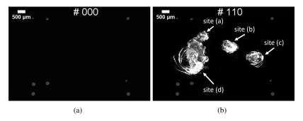
**Fig. 10.** Acquired images of the sample at high resolution (a) before damage growth (# 000) and (b) after the last laser shot (# 110). Four damage sites grew during the growth sequence (see Visualization 1).
