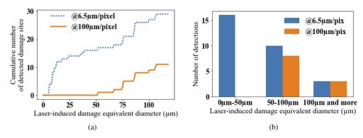
**Fig. 9.** (a) Cumulative number of initiated damage sites detected at high and low resolutions as function of damage site diameter. (b) Number of initiated damage sites detected at high and low resolutions as functions of damage site diameter.
