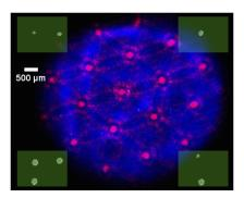
**Fig. 3.** Composite image depicting the observed area of the fused silica sample by the high resolution camera. Initiated laser markers are displayed in light green. The area used for image registration purposes is represented as green boxes. The damage initiation beam is shown in magenta. The damage growth beam is shown in blue.
