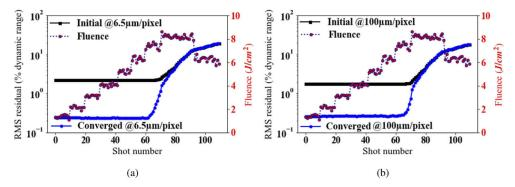
**Fig. 8.** Mean fluence of the shots inducing damage initiation and growth. RMS residuals obtained before and after image registration and laser beam fluence (a) at high resolution (6.5  $\mu$ m/pixel) and (b) low resolution (100  $\mu$ m/pixel).
