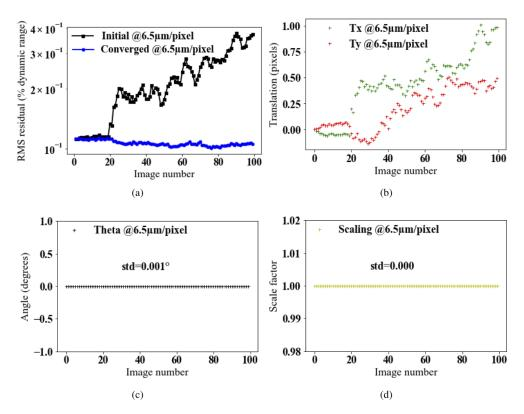
**Fig. 4.** Measurement results for the image set at high resolution (6.5  $\mu$ m/pixel) to estimate uncertainties. (a) RMS residual between the reference image 0 and all images of the set before correction and after image registration. Measured translations (b), rotations (c) and scale factor (d) as functions of image number.
