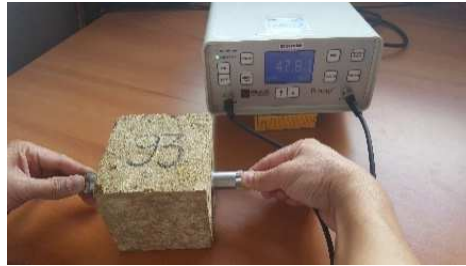
Figure 6: Measurement of the Ultrasonic Pulse Velocity
