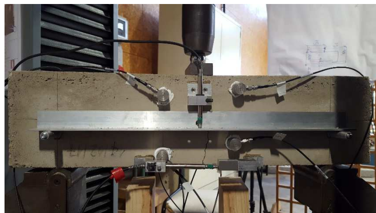
Figure 5: General view of the three-point bending test on soil concrete beams
