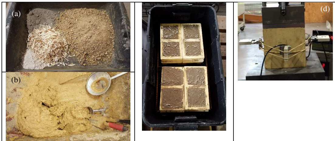
Figure 4: General view of the casted concrete, a) dry materials, b) fresh soil concrete, c) fresh concrete in cubic molds d) compressive test setup on cubic soil concrete (d)
