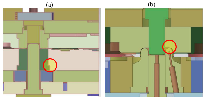
Fig. 9: The position of the thermocouples on the Dies for the two steps: (a) step-1, (b) step-2.
