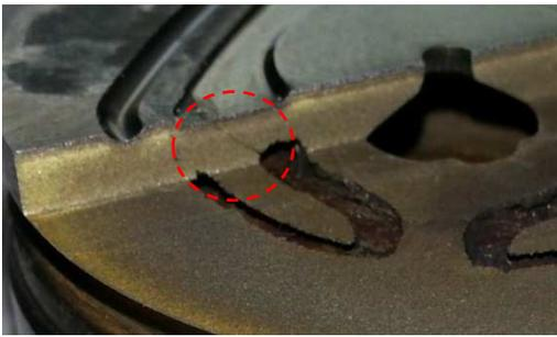
Fig.11. Crack initiation due to high roughness of SLM built conformal channel surface (Courtesy of IPC).
