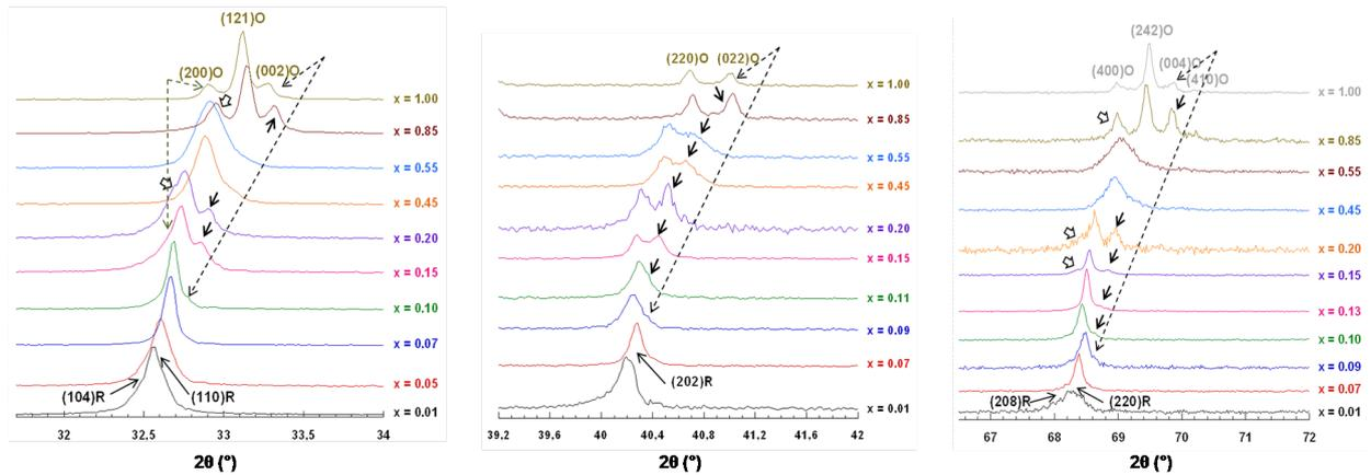
Figure 5: Evolution of XRD peaks of the (1-x)NBT-xCT solid solutions near the MPB region (without the contribution of  $\text{CuK}\alpha_2$ ) in the magnified range  $2\theta$  ( $32^\circ$ - $34^\circ$ ), ( $39.2^\circ$ - $42^\circ$ ) and ( $67^\circ$ - $72^\circ$ ). The arrows indicate the appearance of two phases and the structural transition  $R3c$  to  $Pnma$  at room temperature. Part of this figure  $2\theta(67^\circ$ - $72^\circ)$  has been reproduced from our previous work [27].
