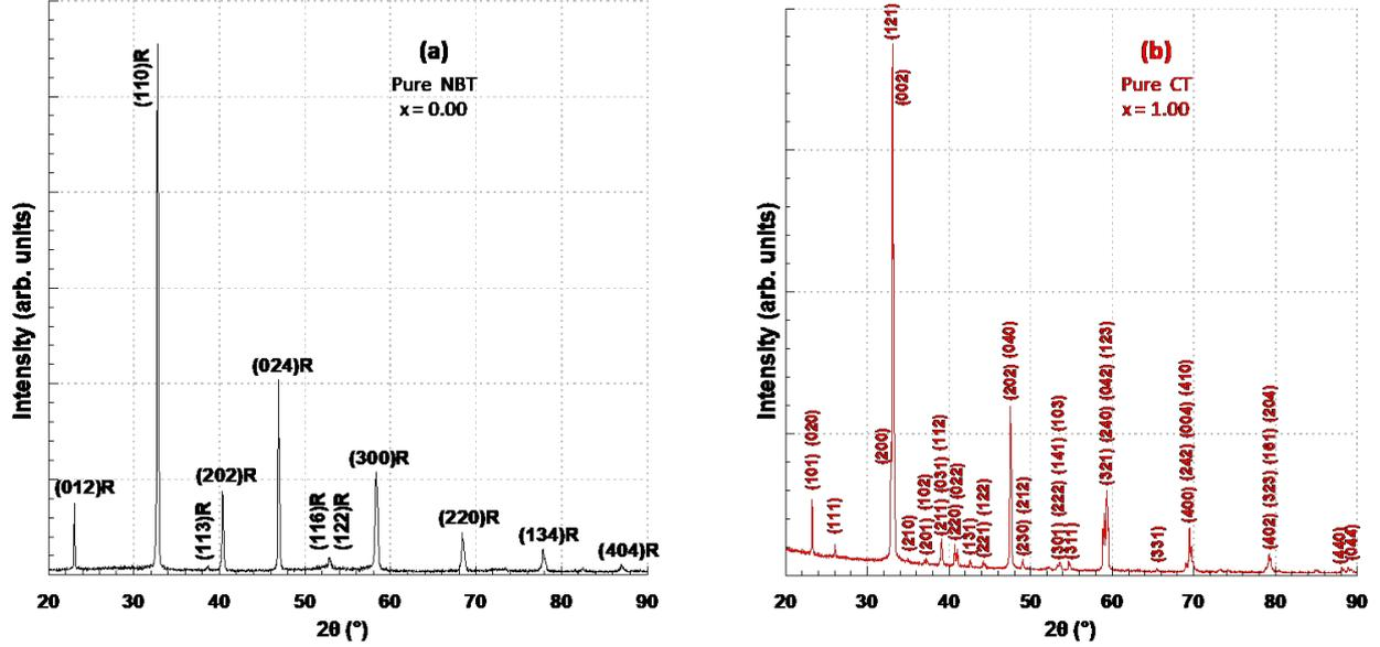
Figure 4: X-ray diffraction patterns of (a) pure NBT ( $x = 0.00$ ) and (b) pure CT ( $x = 1.00$ ) solid solutions at room temperature.
