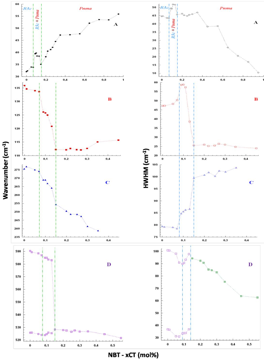
Figure 3: Variation of wavenumber (frequency position) and their corresponding half-width at half maximum (HWHM) of individual bands as a function of x composition for (1-x)NBT – xCT solid solutions at room temperature. Dashed lines are benchmarks to better visualize discontinuities and slope changes associated with phase transitions.
