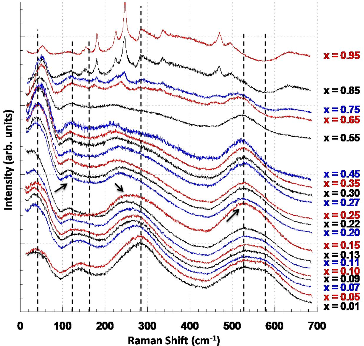
Figure 2: Evolution of Raman spectra for  $(1-x)\text{NBT} - x\text{CT}$  solid solution as a function of  $x$  ( $0.01 \leq x \leq 0.95$ ) at room temperature.
