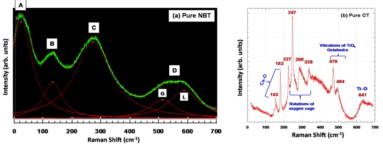
Figure 1: (a) Room temperature deconvoluted Raman spectrum of pure NBT solid solution according to five modes (Lorentzian and Gaussian) and (b) Raman spectrum of pure CT at room temperature.
