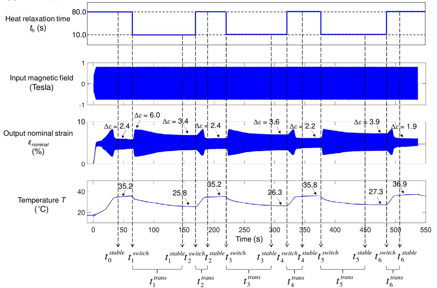
Figure 6. Cyclic transitions of different stable states driven by switching the ambient heat-transfer efficiency (a) Scheme (I) with cyclic switching  $t_h$  between 10.5 s and 8.0 s, (b) Scheme (II) with cyclic switching  $t_h$  between 80.0 s and 25.0 s, and (c) Scheme (III) with cyclic switching  $t_h$  between 80.0 s and 10.0 s.
