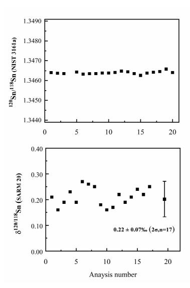
Fig. 2 Analytical precision of standard solution of NIST 3161a and coal standard SARM 20
