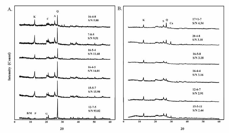
Fig. 3 XRD spectras of the coal samples. The intensities of the samples were normalized basing on sample #12-7-5. The samples were classified into two groups by their calculated S/N. A) Group Min, B) Group Org.
