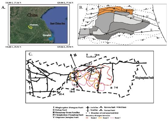
Fig. 1 A) Location of Huainan Coalfield, B) Main faults in Huainan Coalfield, and C) Locations of minor faults and sample drilling holes, and magma intrusion boundaries of coal seam No.4, No.5 and No.7 in Zhuji Coal Mine, Huainan Coalfield
