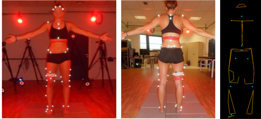
Figure 2: Markers and EMG sensor placement for the static posture of participant 7. From left to right: anterior and posterior views, and a visualisation using MOKKA software of experimental markers (linked by yellow bars) and calculated joint centres (represented in blue). The markers placed on the left tibia were removed for stretching tests.
