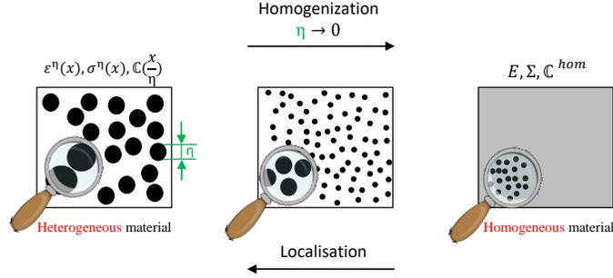
**Fig. 1.** Principle of asymptotic expansion homogenization method.
