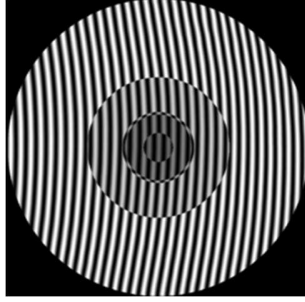
Fig. 8. The hologram of Fig. 3 after including the phase correction term \phi_c to compensate the aberrations introduced by the LCoS.
