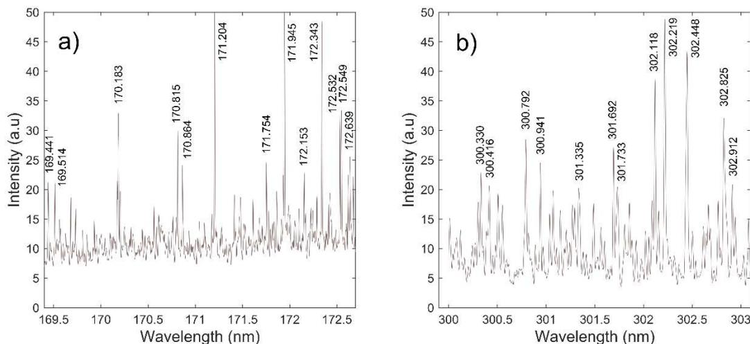
Figure 3 : ICP-OES spectra of a 1g/L uranium solution in the VUV (a) and UV-visible (b) ranges. The spectrum of the solvent has been subtracted. Labels show the wavelength of the most intense observed lines.
