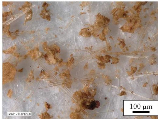
Fig.15 Optical microscope image of wear debris in grease
