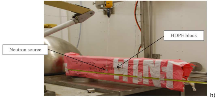
Fig. 3a) Schematic representation of the experimental protocol, and b) experimental setup with distance-operated screening of the neutron source.
