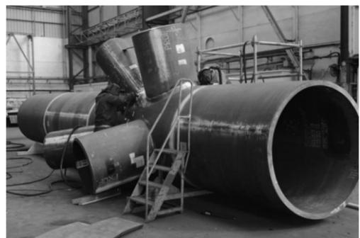
Figure 2: Stress computation points around the circumference of a welded tubular joint and Jacket structure realized by Atlantique Engineering Solutions for Alstom offshore prototype Haliade 150 (photo courtesy of Bernard Biger)
