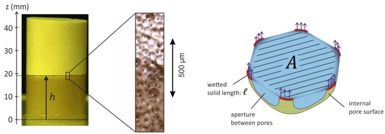
The measured rise velocity of liquid in solid foam is one order of magnitude smaller than the predicted value. This deviation is attributed to the excess time spent by the liquid-gas interface at connections between pores.
