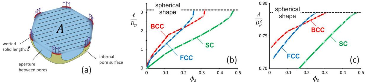
**Fig. 6:** (a) Sketch of single representative foam pore (cut at the middle cross-section for clarity). In each pore, surface tension acting at the solid surface (shown by the arrows) supports the column of liquid beneath the interface. (b) Wetted solid length  $\ell$  divided by  $D_p$  as a function of solid volume fraction for three ideal foam structures: FCC, BCC (Kelvin) and SC. (c) Pore cross section  $A$  divided by  $D_p^2$  for three ideal foam structures: FCC, BCC (Kelvin) and SC.
