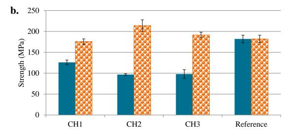
Figure 13: Composite mechanical properties estimated at  $V_f = 45\%$  (Reference = flax cross-ply laminate)
