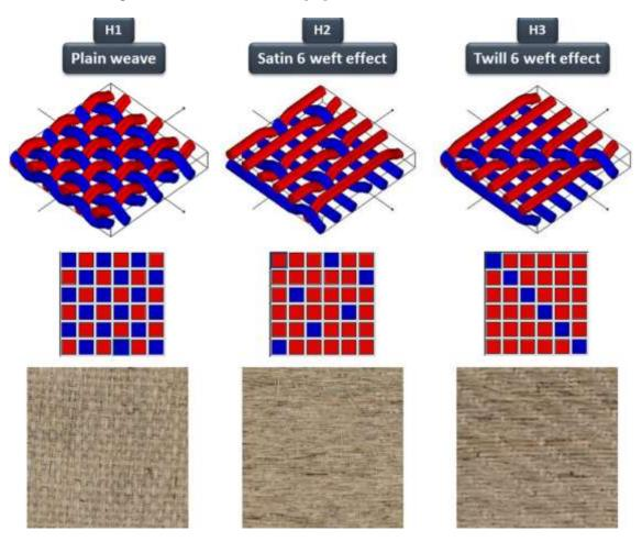
Figure 1: Schematic representation and pictures of the woven fabrics manufactured and studied in this
