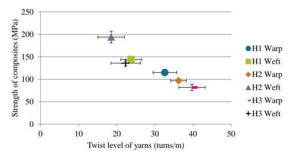
Figure 14: Relationship between the twist level of the rovings in the fabrics and the strength of
