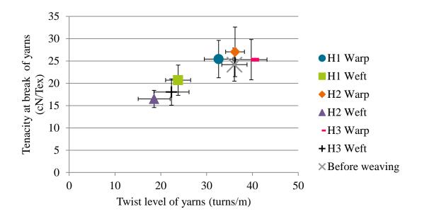
Figure 7: Breaking tenacity of the rovings as a function of their twist level. Evidence of a direct
