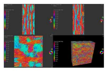
Figure 10: Nanotomography views of CH2 composite
