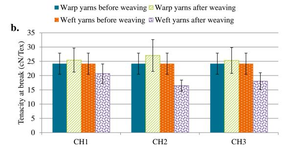
Figure 6 : Influence of weaving process on yarns properties a. Twist level b. Tenacity at break
