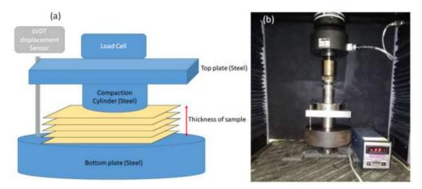
Figure 2: Compaction test setup a. schematic diagram with preforms b. configuration for machine
