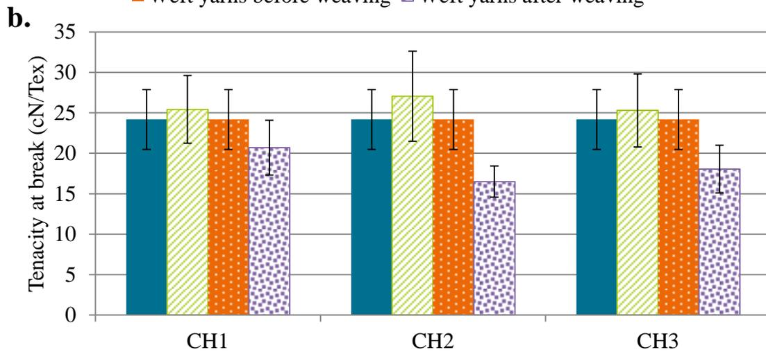
Figure 6 : Influence of weaving process on yarns properties a. Twist level b. Tenacity at break
