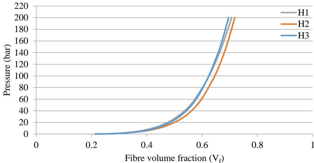
Figure 5: Compaction curves for the three hemp fabrics
