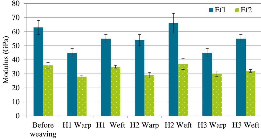
Figure 8: Comparison of the fiber stiffness before and after weaving for the three considered fabrics
