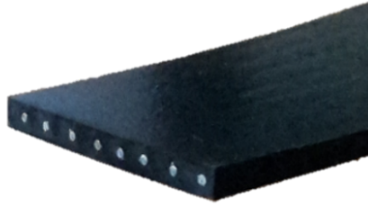
Figure 2: Transverse cut of a composite specimen
