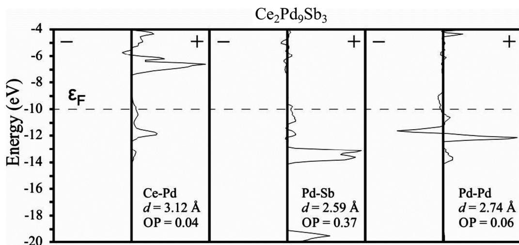
**Fig. 4.** EH *COOP* curves of representative bonds in  $\text{Ce}_2\text{Pd}_9\text{Sb}_3$ . The + region is the bonding area and the - region the antibonding area. The bond type, distance and integrated overlap population up to the Fermi level are indicated in each panel.
