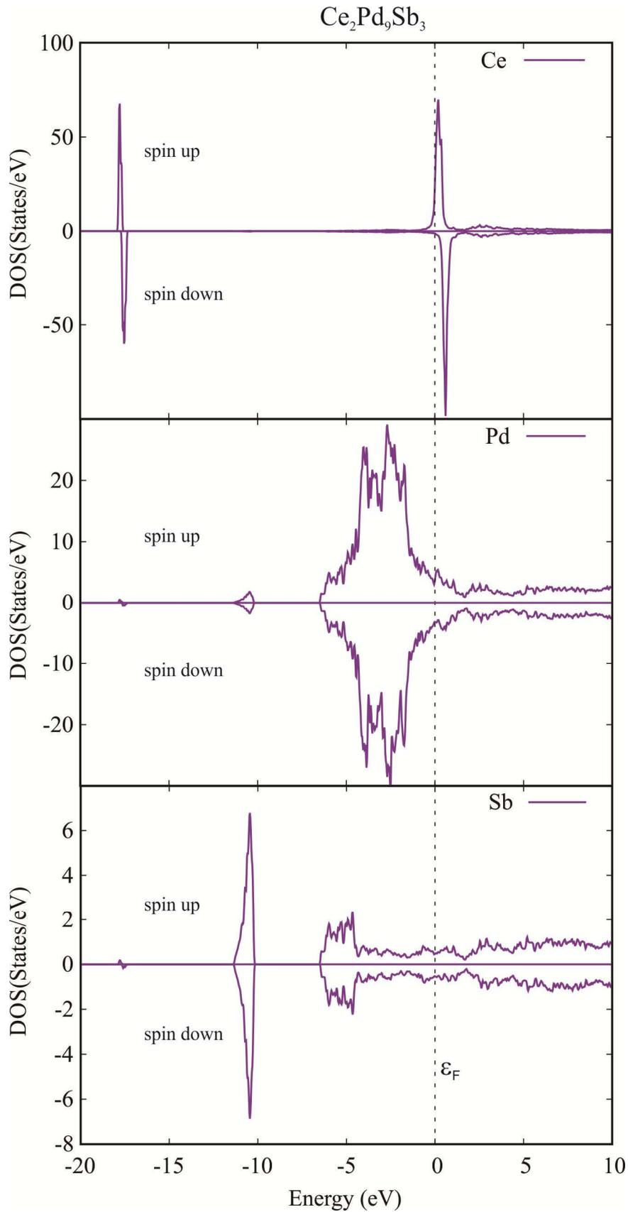
**Fig. 5.** Spin-polarized DOS of  $\text{Sm}_2\text{Pd}_9\text{Sb}_3$  calculated by the WIEN2k package. The upper panel is the total DOS of Sm, most of it is Ce 4*f* near the Fermi level. The middle one is the total DOS of Pd, most of it is the 4*d* of Pd. The lower panel is the total DOS of Sb.
