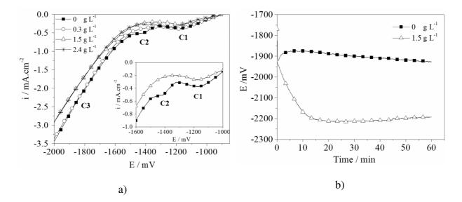
Fig. 1. Cathodic polarization curves (scan rate:  $1 \text{ mV s}^{-1}$ ) (a) and chronopotentiometric curves at i = -3 mA.cm<sup>-2</sup> (b) of steel in supporting electrolyte without Zn<sup>2+</sup> ions with different NE concentrations.
