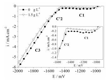
Fig. 4. Cathodic polarization curves of steel in the plating bath (with  $Zn^{2+}$  ions) without and with 1.5 g L<sup>-1</sup> NE (scan rate: 1 mV s<sup>-1</sup>).
