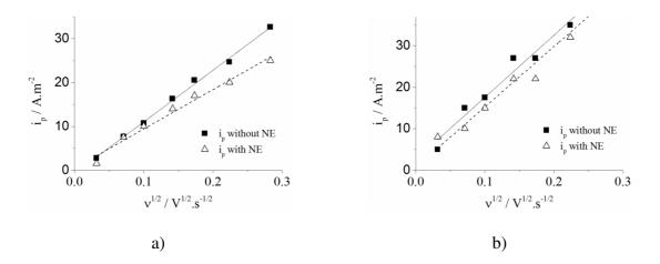
Fig. 6. Cathodic peak current  $(i_p)$  of the cathodic peak C1 (a) and C'2 (b) as a function of the sweep rate without and with 1.5 g L<sup>-1</sup> of NE.
