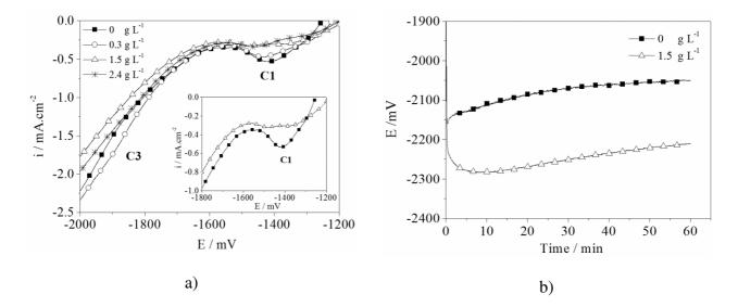
**Fig. 3.** Cathodic polarization curves (scan rate: 1 mV s<sup>-1</sup>) (a) and chronopotentiometric curves at i = -3 mA.cm<sup>-2</sup> (b) of zinc in supporting electrolyte without Zn<sup>2+</sup> ions with different NE
