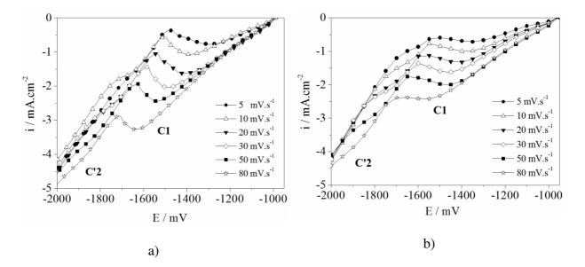
Fig. 5. Effect of potential scan rate on the cathodic polarization curves of steel in the plating bath (with  $Zn^{2+}$  ions), without (a) and with 1.5 g L<sup>-1</sup> of NE (b).
