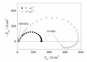
Fig. 2. Nyquist diagrams of steel in supporting electrolyte without  $Zn^{2+}$  ions without and with 1.5 g L<sup>-1</sup> NE at open-circuit potential.
