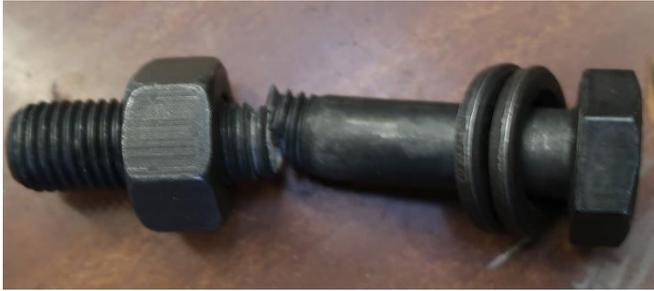
a- Bolt rupture in tension
