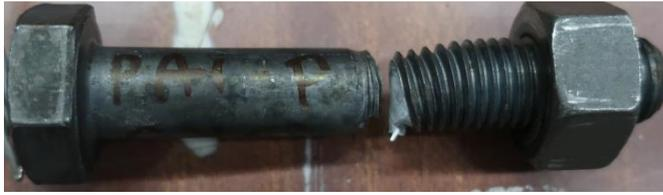
*a- Bolt rupture in tension*
