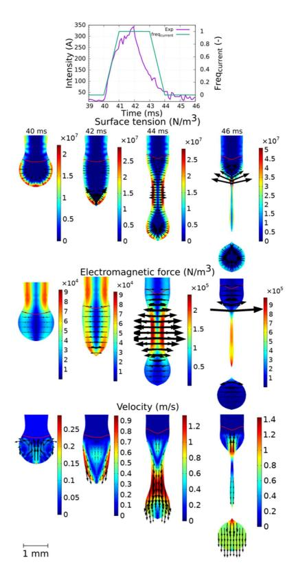
Fig. 7 - A sequence of the distribution of calculated process variables showing different moments during a pulse cycle
