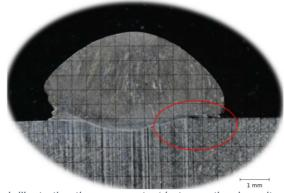
Fig. 13 – Macrograph illustrating the poor contact between the deposit and the substrate
