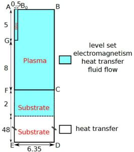
Fig. 1 - Geometry of the model (dimensions in mm)
