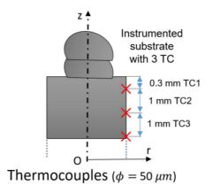
Fig. 4 - Diagram illustrating the positioning of the thermocouples
