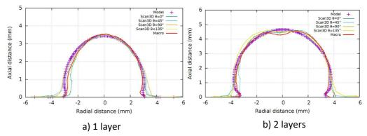
Fig. 11 - Comparisons of the profiles of the deposits from the model with those of the 3D scan and the macrographies for one layer (a) and two layers (b)
