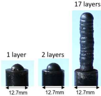
Fig. 3 - Photographies of different rods obtained with pulse WAAM
