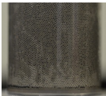
Figure 5: Bottom of cement foam sample 15 minutes after production (TTAB, R = 300 \mu\text{m} , W/C_f=0.69 with perfluorohexane). Sample diameter is 2.6 cm.
