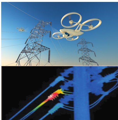
(b) UAV-based power lines inspection [58, 3].
