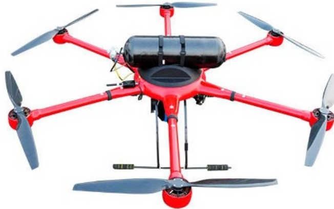
Figure 18: MMC's HyDrone 1550 multicopter equipped with 1800W H1-Fuel Cell [117].
