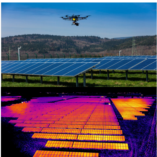
(a) UAV-based solar photovoltaic panels inspection [56, 57].
