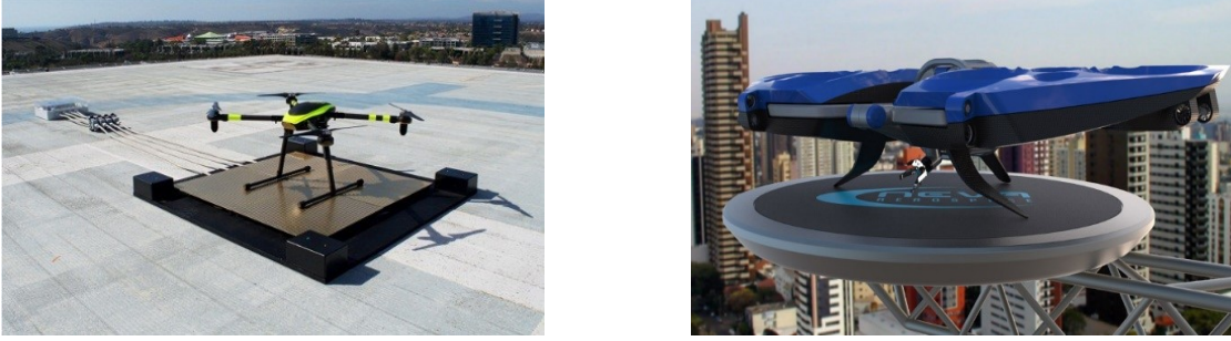
Figure 15: UAV's charging stations [96, 101].
