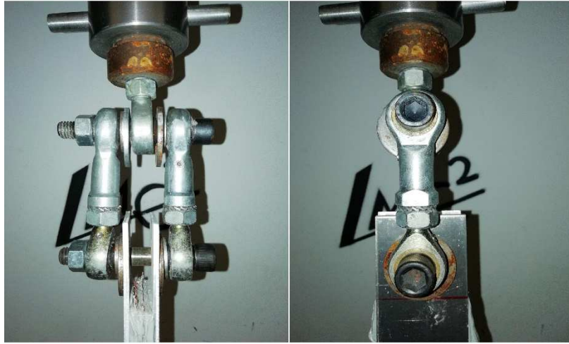
Fig. 3: Ball-joint loading heads used to transmit the load from the Zwick press to the TRCMC specimen.
