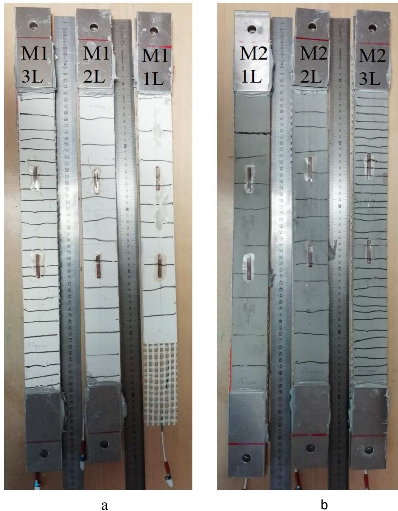
Fig. 14: Cracking diagram of specimens after tensile tests with three reinforcement ratios (L denotes layer): (a) Matrix M1 and (b) Matrix M2.
