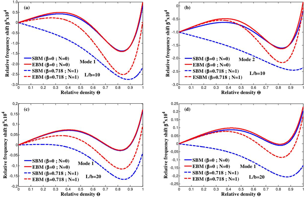
**Fig.6.** The frequency shift versus  $\Theta$  obtained for the full  $(\beta,N)=(0,0)$  and perforated  $(\beta,N)=(0.718,1)$  systems with  $h=10nm$ :  $L/b=10$  for (a) mode 1 and (b) mode 2;  $L/b=20$  for (c) mode 1 and (d) mode 2.
