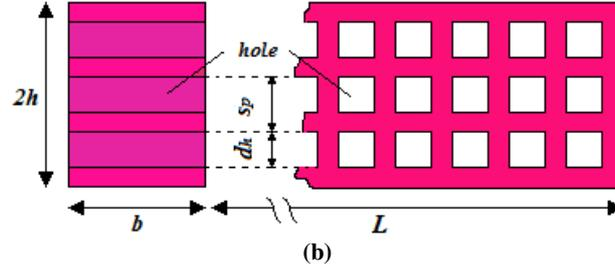
**Fig.1.** The model of the adatom-nanobeam system: (a) The perforated nanobeam structure containing adatoms distributed on its upper surface and (b) the geometry of the perforated nanobeam structure containing aperiodic square hole network.
