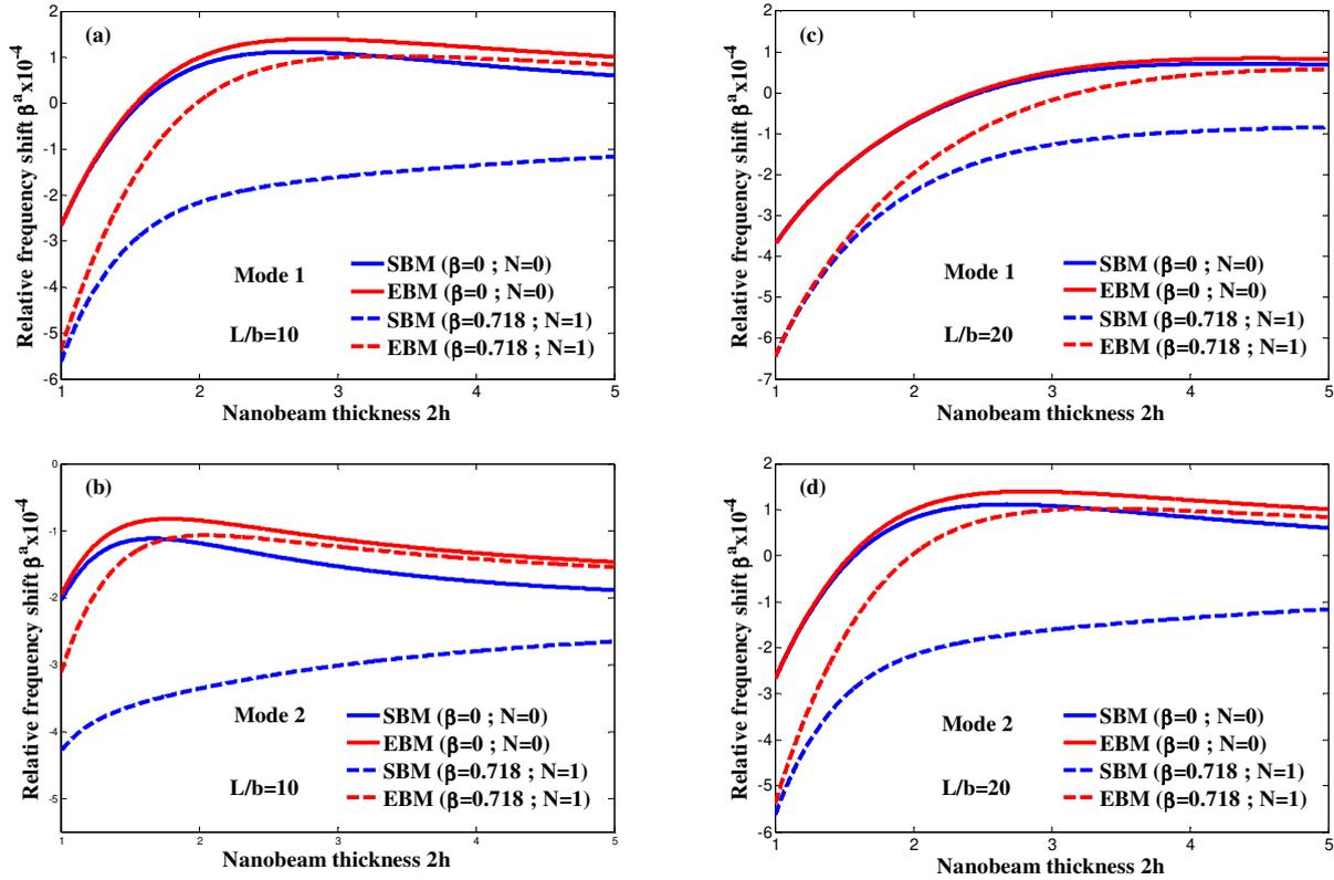
**Fig.5.** The frequency shift versus thickness ( $2h$ ) for the full  $(\beta, N)=(0, 0)$  and perforated  $(\beta, N)=(0.718, 1)$  systems with  $\Theta=1$ :  $L/b=10$  for (a) mode 1 and (b) mode 2;  $L/b=20$  for (c) mode 1 and (d) mode 2.
