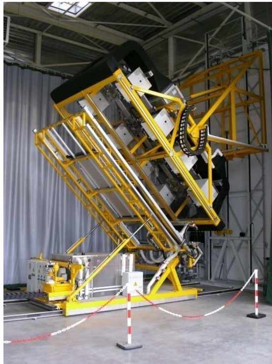
Fig. 3. Indoor test stand for solar thermal collectors.
