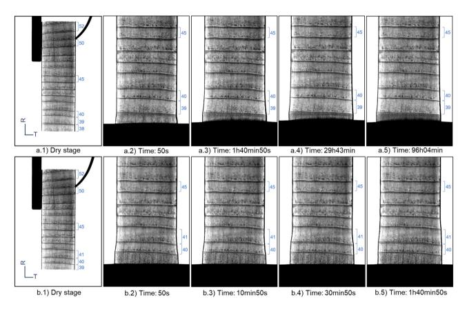
Figure 9: Water uptake in Norway spruce along the radial direction at several different times: (a) in the first test (including Ring #38) and (b) in the second test (after removing the Ring #38).
