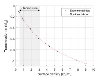
Figure 3: Experimental data from Sorbus samples of different thicknesses and moisture contents with the non-linear fitting curve (Equation (5)). The range of surface densities used later in this work is represented in grey.
