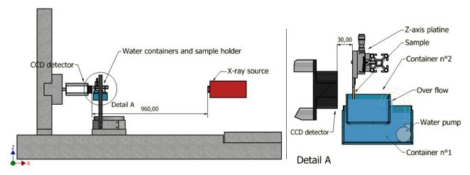
Figure 1: Scheme of the experimental setup of 2D X-ray imaging.
