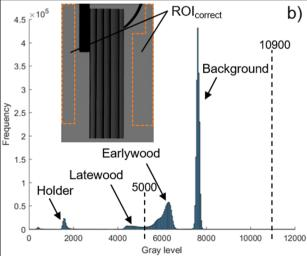
Figure 2: Distribution of grey level before (a) and after (b) image processing. Vertical dashed lines represent the limit of brightness and contrast of the inset image.
