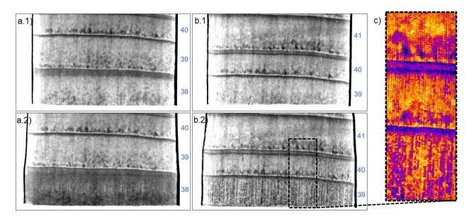
Figure 10: Bottom of the sample before (subscript 1) and at the end (subscript 2) of the first imbibition experiment (a) and second and (b). c) Zoom on the area pointed out by the dashed line, with the LUT "Fire".
