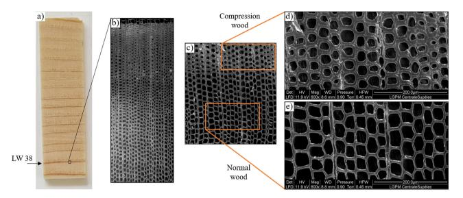
Figure 12: ESEM images of the annual ring of interest 38 from twin sample (photography) used for imbibition experiment in radial direction.
